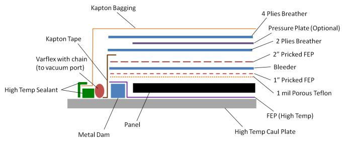
Figure 2 | Alternate Bagging Scheme for CYCOM 2237
